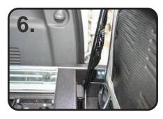
Squeeze handle trigger to disengage and return to upper position, depress slide lock and push handle to return Easy Slide to stowed position. Engage the Transit Lock by sliding the lever to the left.
